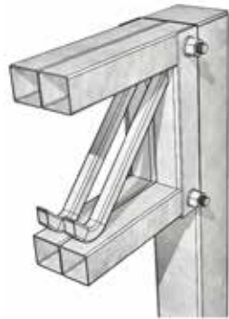
2 HB Double HB - to Column (shoe welded to column by Hopleys)
