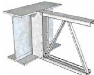
10 HJ Vertical hung shoe to suit nominated structural UB/UC (weld on site)
