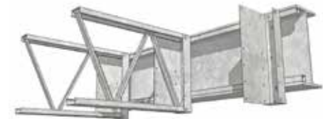
12 HJ Smaller Beam with vertical SHS Stubs welded to flanges by Hopleys or Steel fabricator
